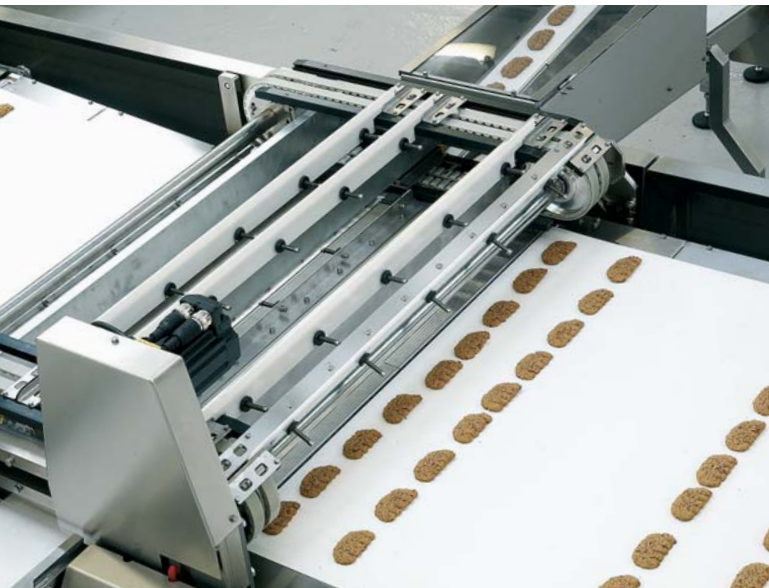
Automatic Distribution System
